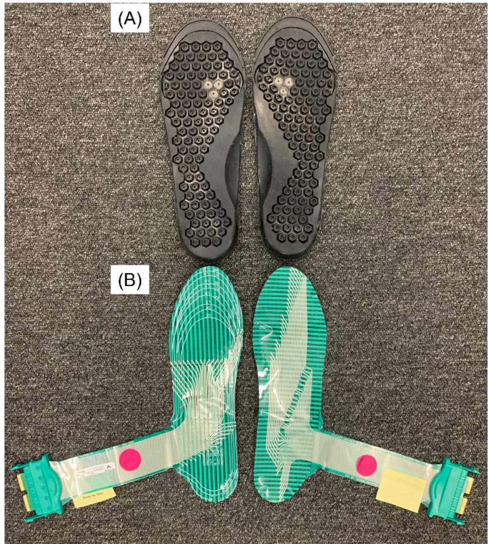
Fig. 1 Experiment setup of (A) bottom view of the prototype insoles with a triangle cavity on each side at the second MTP joint, (B) F-Scan insoles for measuring plantar pressure
